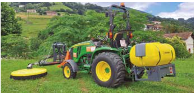
S-dome 1200 sprayer with hydraulic structure (5-7m) and 300L tank
