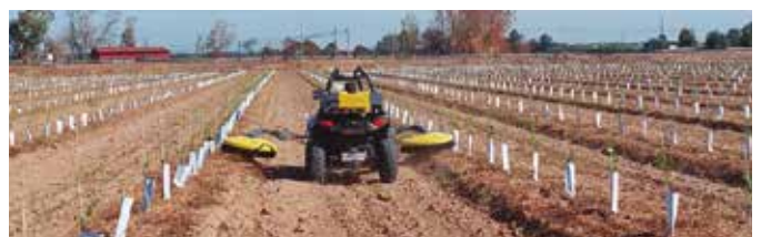
S-dome 900 sprayer with electrical structure in young almond plantation 3.6 x 1.2m
