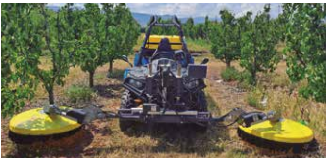
S-dome 900 sprayer with electrical structure, in pear and peach trees, 4 x 1.5m
