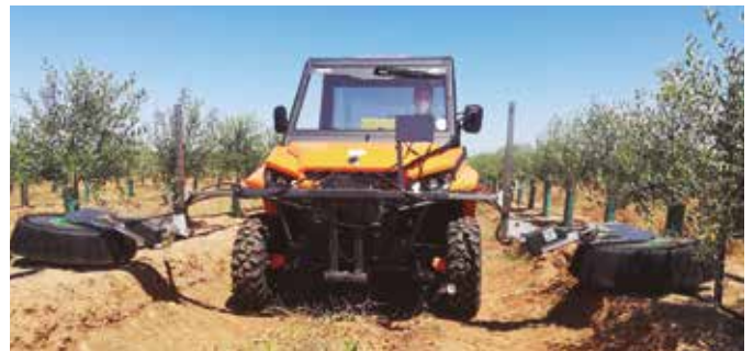
S-flex 400 sprayer with manual structure, vineyards 2.3 m
