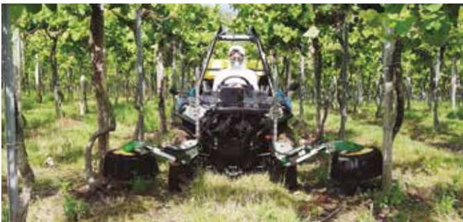
S-flex 600 sprayer with manual structure, olives 4 x 1.5m
