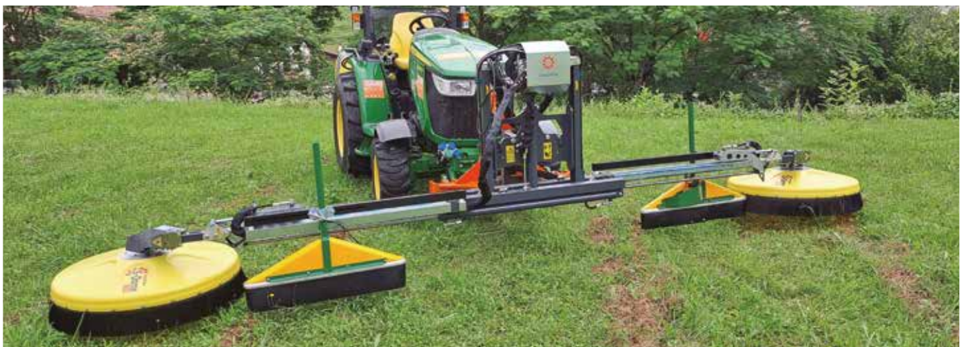
S-dome 1200 and S-miser with hydraulic structure, for 7m row width and 2m band width.
