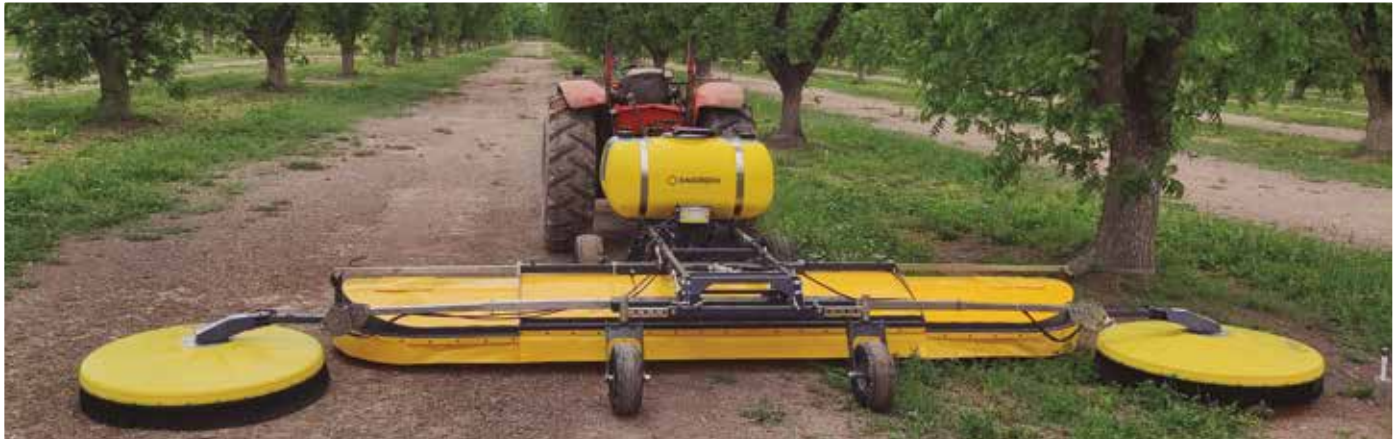
S-dome+ 3049 with S-dome 1200 shields (7.2m width treatment), walnut trees 12x12m
