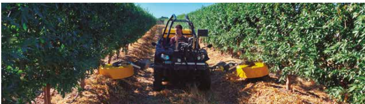
S-flex 600 sprayer with vinyl covers and manual structure, almonds 3,6 m
