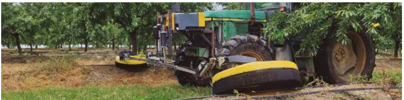
S-dome 900 sprayer with electrical structure and 60L tank, almonds 6 x 6m
