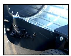
Chain tension adjustment and low maintenance bearings.
