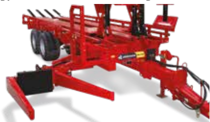
Adjustable loading arm for all types of bales, wet or dry
