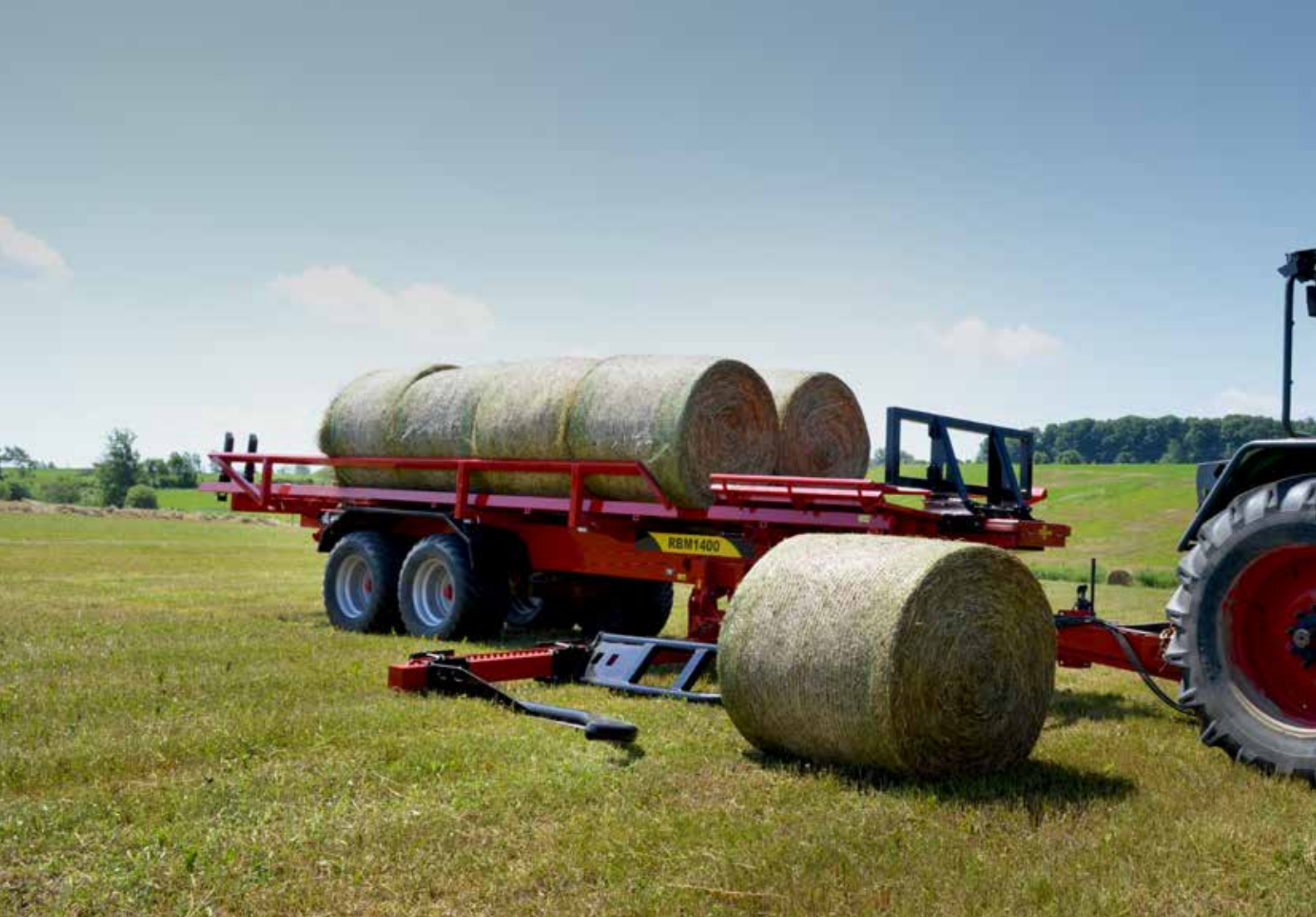
Effortless unloading by continous hydraulic thrust
