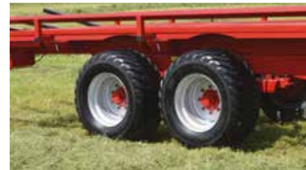
Tandem axle and high flotation tires
