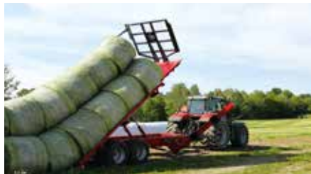
Effortless gravity unloading at 40 degree angle
