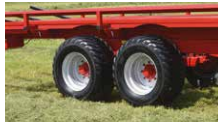
Tandem axle and high flotation tires
