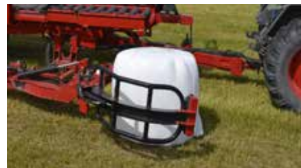
In-Motion loading arm technology
