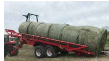
Effortless unloading by continuous hydraulic thrust
