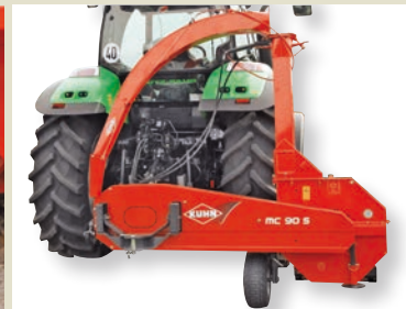
Foldable chute for storage and transport (MC 90 S and MC 90 S TWIN)
