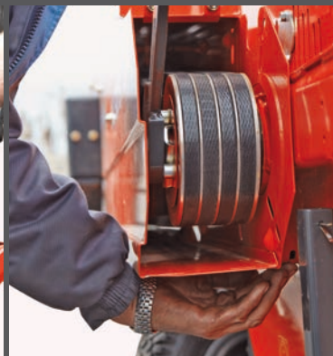
After sharpening the knives the chopping wheel can easily be adjusted
