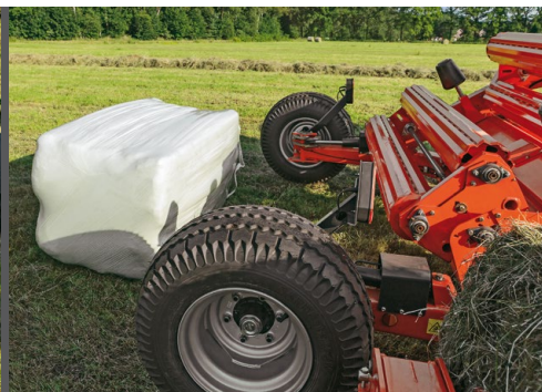
The low table height allows the bale to be gently tipped off to prevent film damage.
