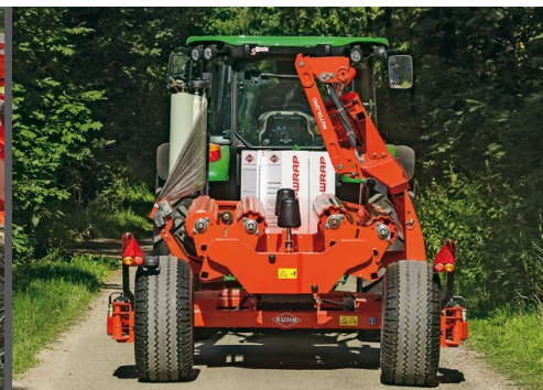
For road transport the wheels can be folded inwards to reduce the transport width. Hydraulic folding is optional.
