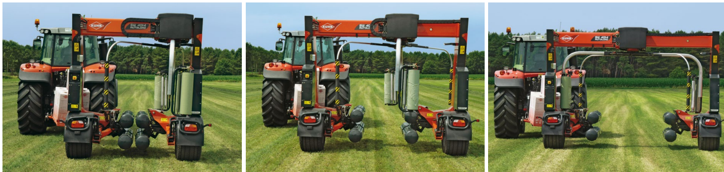
The wrapper folds from its 2,5 m transport position into 4 m wide field position.
