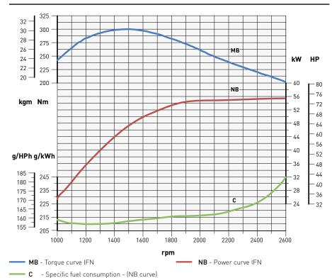
Power ratings refer to engines equipped with air filter, standard muffler, after running-in period at ambient conditions of +25°C, relative humidity 30% and 1 bar. De-rating depending on applications.
