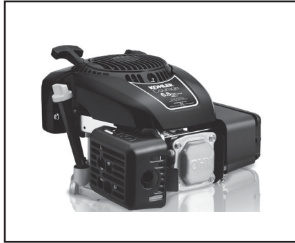
XT Series 6.5-7.75 ft-lb Gross Torque Air-cooled, vertical, OHV Models: XT650, XT675, XT775
