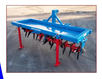
The **GROW-MASTER** is available in 2.0m, 2.4m, 2.8m and 3.2m working widths. Horse-power requirement is quite low with a minimum of only 35Hp required for the 2.0m unit. A tow hook is mounted on the back for dragging pasture harrows. Harrow carriers are also available on request.
