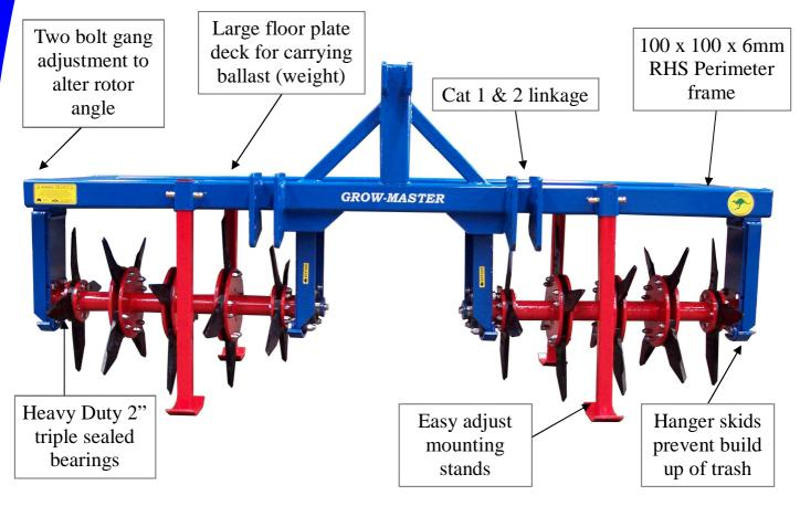
Designed specifically for the sugar cane industry, this 2.5m aerator straddles the cane with each rotor aerating the outer track. Each rotor consists of 5 rows of 4 tines spaced 200mm apart. The outer 2 rows are approximately 60mm higher than then centre 3 rows. This prevents damage to the cane runners on the edge of the row. The centre tines are positioned for 1650mm row spacings.
