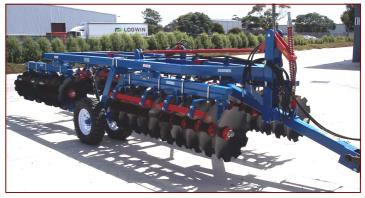
Picture above: 40 plate model shown fully closed up for transport
