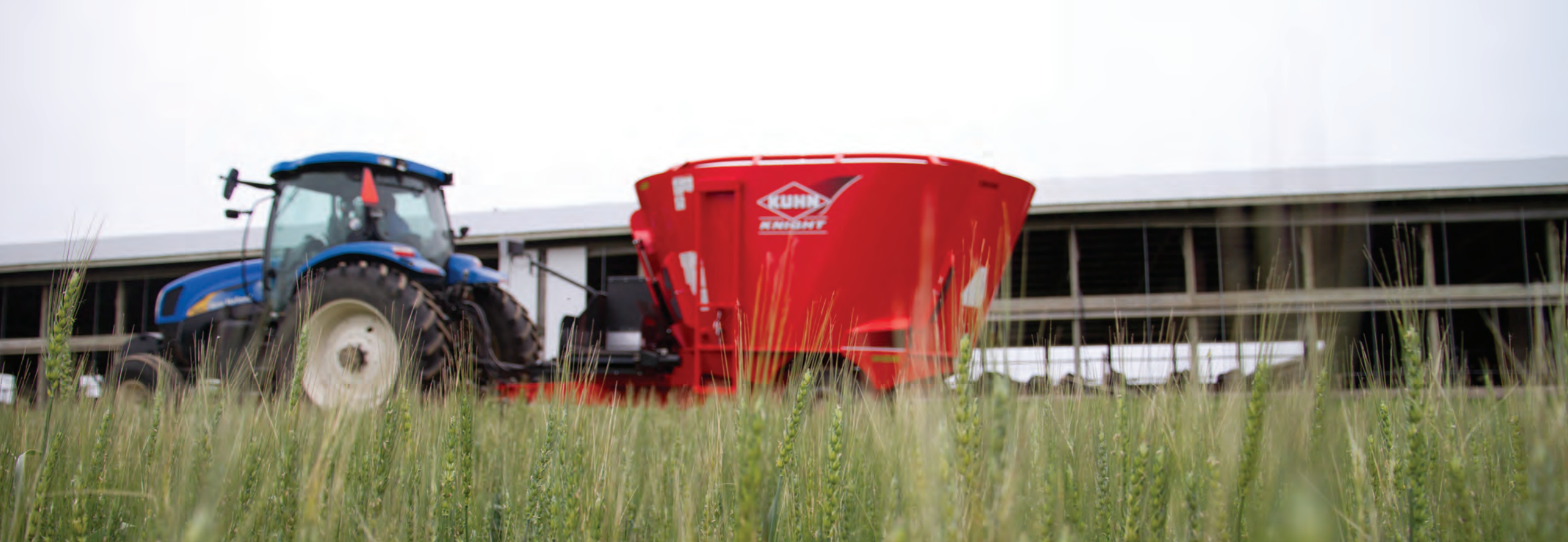
HEAVY-DUTY, SINGLE-AXLE TRAILER The single axle, dual-wheel design allows for ease of maneuverability, reduced ground pressure and overall stability. Both implement and truck tires are available.
