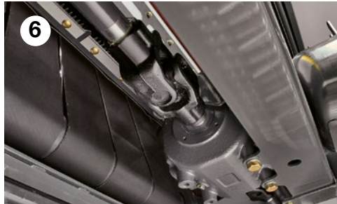
6 Heavy duty cross joints in the drive axles
