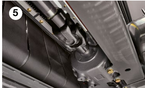
5 Heavy duty cross joints in the drive axles
