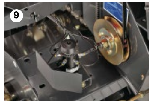
9 Beka Max continuous chain oiling system
