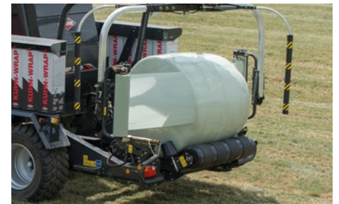
Switches to conventional wrapping for 100% film coverage.
