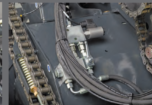
Separate knife/Drop Floor controlled from the tractor seat
