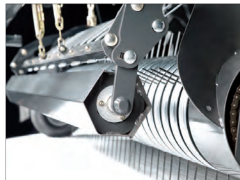
Low-profile, 5-tine bar pickup
