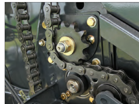
Heavy-duty chains and hardened sprockets
