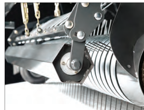
Low-profile, 4-tine bar pickup
