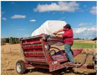
The loading system suspends the bale above the feeding deck to simplify the removal of net and plastic and wrap.
