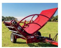
The feed platform is raised and lowered by the operator to control the feed rate.
