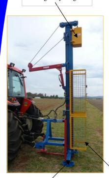
An adjustable sliding clamp is fitted to the main beam to keep post straight when driven
