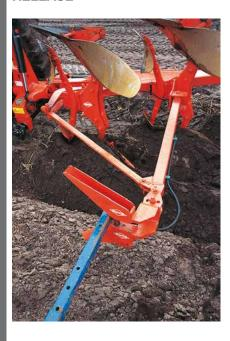
Available for the complete plough range the arm allows the use of a furrow press with easy hooking up and hydraulic push-off. On the pick-up hook part of the arm where there is most risk of damage all grease nipples and hydraulic hoses are protected inside the structure of the head. The arm folds up conveniently for subsequent transport.
