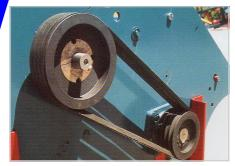
Belt drives lessen the shock loads which mulchers have to endure. Consisting of either 3 or 4 belts, depending on size, they are fitted using taper lock pullies for ease of maintenance (pictured left).
