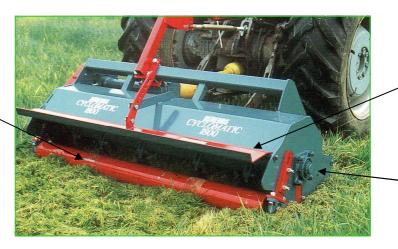
Adjustable back flap doubles as a scraper for the roller when in the mulching position.
