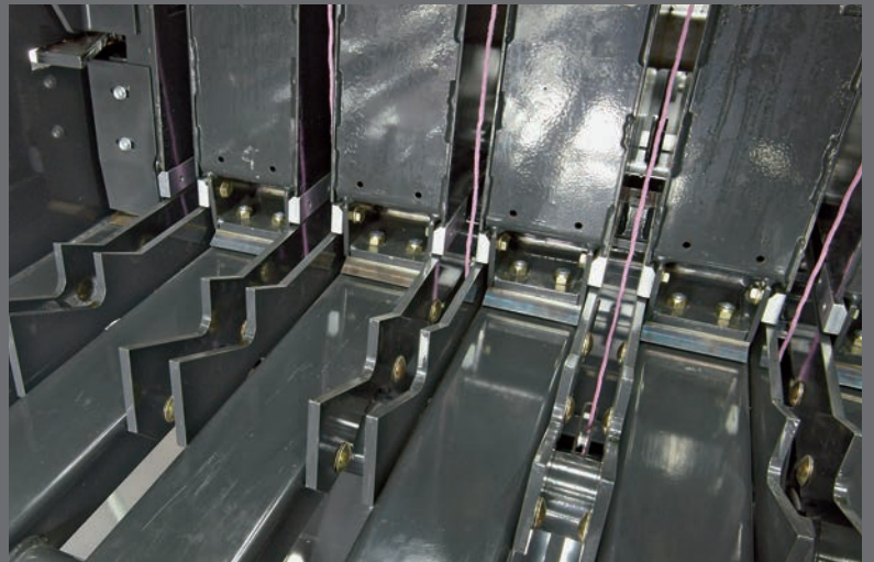
Bottom retainers prevent decompression of the bale and provide extra density
