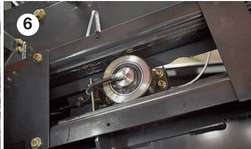
High capacity plunger - 46 strokes per minute 12,5 cm diameter plunger rollers
