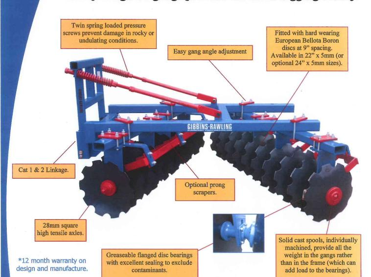
MODEL 18 plate 20 plate 22 plate 24 plate 940kg Approx Weight 820kg 860kg 910kg No. bearings 4 No. axles 2 4 4
