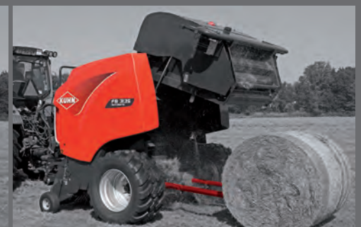
Bale kicker notices when bale is out of reach. The tailgate is not opened any further than necessary. The tailgate closes automatically.
