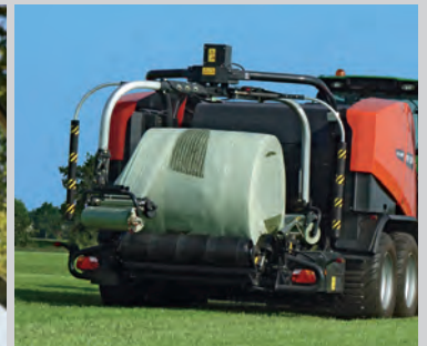
3D wrapping for well-shaped, tightly sealed bales (optional)
