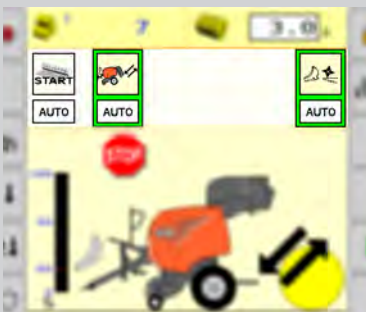
High level of comfort by fully automatic tailgate operation and rotor DEBLOCK system (AUTOMATE function optional for FB 3135)
