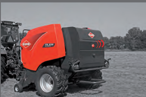
Net binding is being applied, visual and acoustic signals on the baler are activated.
