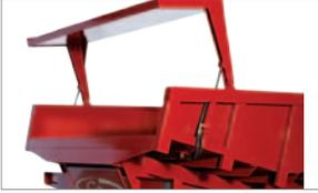
Optional hydraulic rear tailgate with twin double acting rams and an enormous opening clearance of 1.2 metres.
