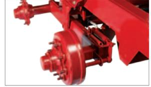
The heavy duty tandem axle is standard with front drum brakes and oscillating beams with replaceable oil impregnated nylon bushes. Large flotation wheels stay on top of the ground, offering traction even on difficult sites.
