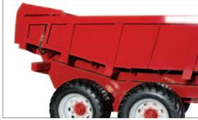
15° rear deck angle keeps material firmly in the trailer, even without a tailgate and gives a high tipping clearance for building stockpiles.
