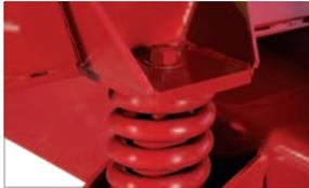
The sprung drawbar reduces shock loading to the tractor towbar, ensuring a smooth power transfer from tractor to trailer and greater operator comfort.
