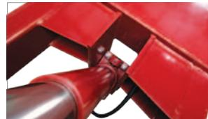
Two way pivot on the multistage ram base eliminates side loads between the stages which can otherwise score the cylinders and damage oil seals.
