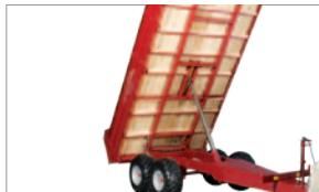
A clever rear pivot design gives high ground clearance and keeps the load centre well forward when the deck is raised, leaving weight on the drawbar. Tipping angles are up to 57° for a clean dump.
