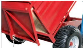
The steel taildoor features a high clearance pivot and adjustable check chains for accurate spreading.
