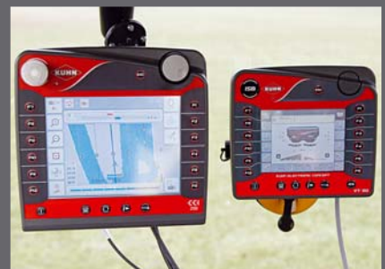
CCI with CCI.Command (Section Control + Parallel Tracking) + VT 50 (machine display)
