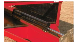
**PIGGYBACK HYDRAULIC CYLINDERS**This unique cylinder design provides smooth and
